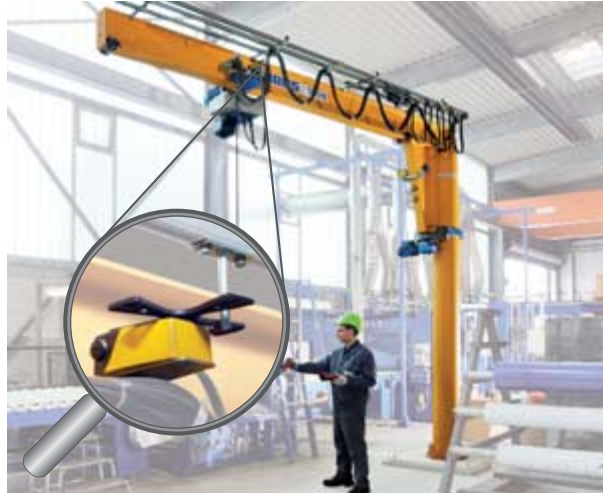
Limit switch for trolley travel (Fig. 8)
