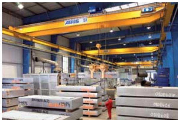
Type D crab units on double-girder overhead travelling cranes
